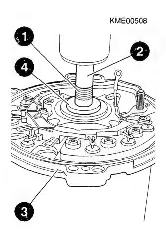
Dismantling windingless rotor
